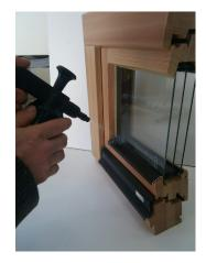
Spray supplied separating gent onto the silicone bead with sparay bottle
