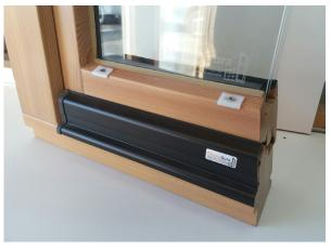
Fix clips 50mm from the sash inside edge and all other clips 200mm centers. Make sure the clip is correctly positioned and in line with the others
