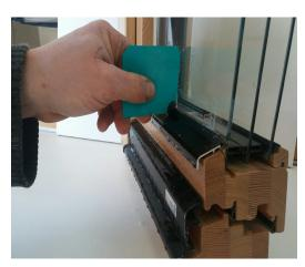
Use the 7mm bevel on the silicone pad to clean off the silicone bead to achieve a nice finish. Pull the pad along the silicone bead. If necessary, spray separating agent again and clean again.
